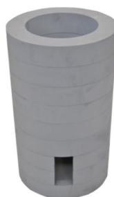
Specs: Lead Rings 12" outside diameter 19 3/4" overall height 575 lbs 2" x 4" cutout in bottom rings for cable
