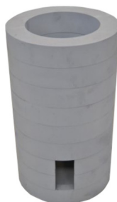
Includes Stainless Steel Cover Specs: Lead Rings Outer Dimensions: 12" Dia x 19.75" H Inner Dimensions: 8" Dia x 17.75" H 575 lbs 2" x 4" cutout in bottom rings for cable
