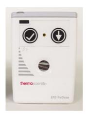
The EPD TruDose Electronic Personal Dosimeter monitors Gamma and Beta radiation in any environment where workers need to monitor their exposure to radiation.
