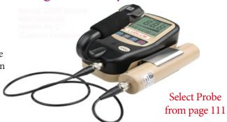
The DMS-3000 is a versatile, lightweight, ergonomically-designed instrument used with an external detector for Alpha, Beta, or Gamma radiation survey. Three modes of operation – RATE, MAX, and COUNT – are available for the user. Measurements can be collected in two sets of units (primary and secondary) for RATE and MAX modes in cps, cpm, Bq, dpm, mR/hr, or µSv/h units. The user can switch between two sets of chosen units by simply pressing the Units button.
