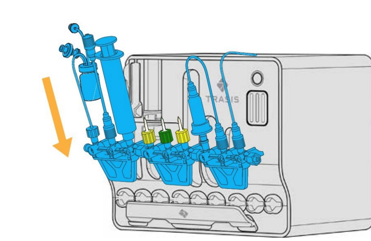
Tilt up the cassette and snap it in place. It automatically locks. Plug the colored coded vials on the matching positions.
