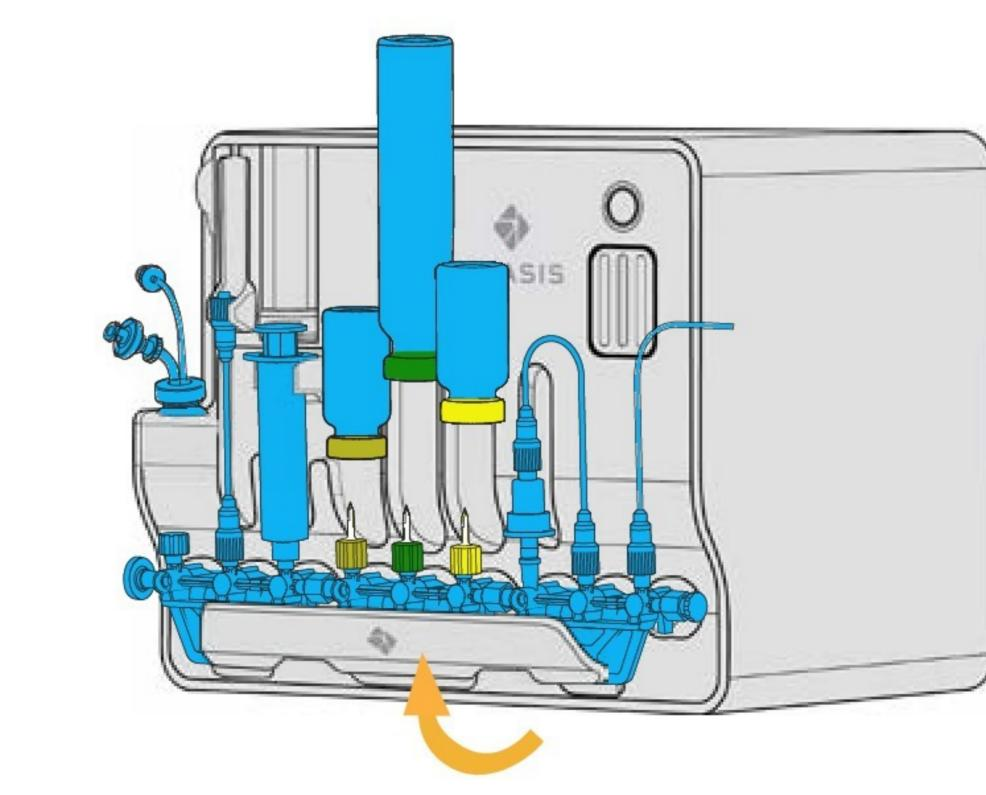
Insert the RFID labels in the slots. EASYONE is ready to start!
